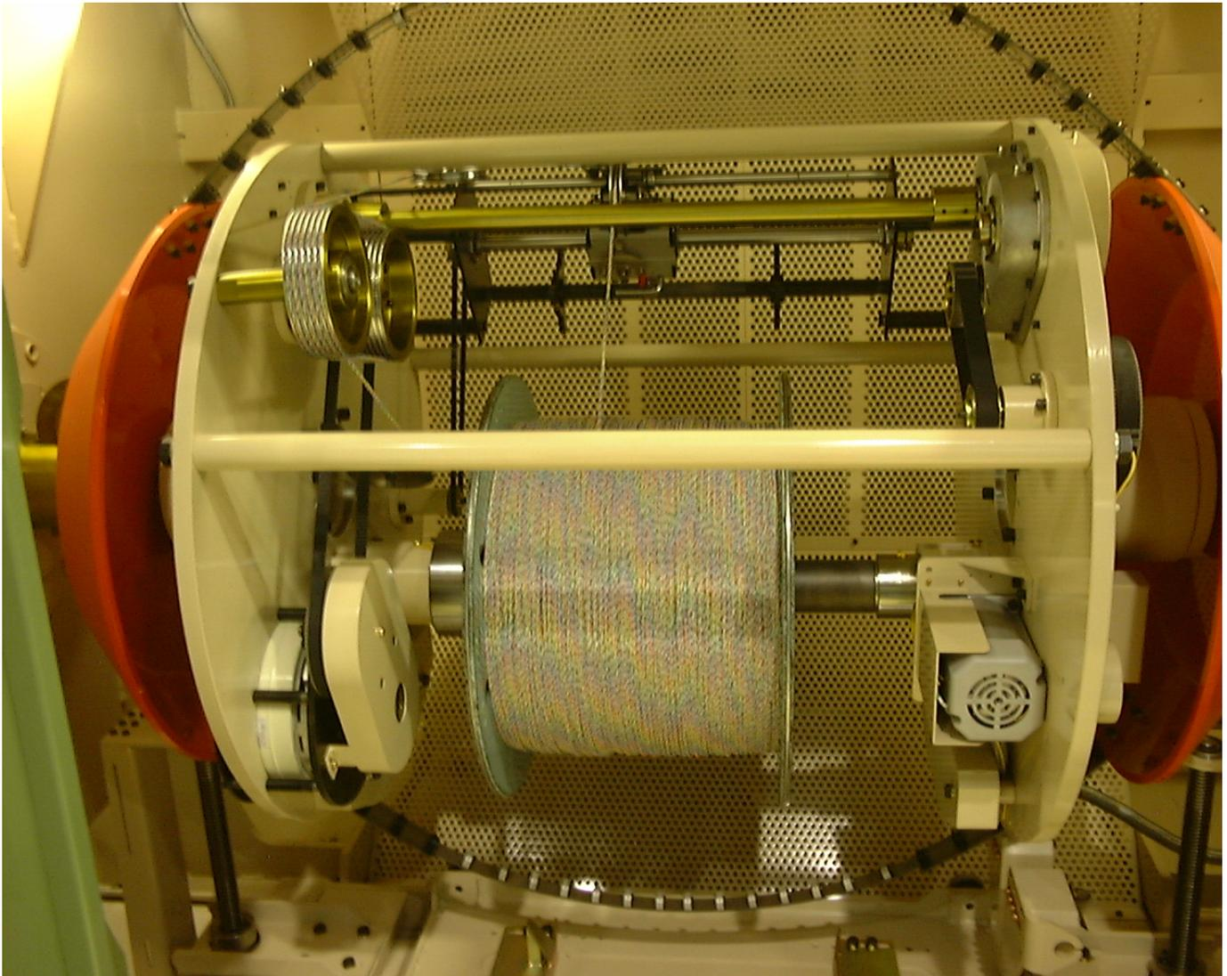
**High performance double twist cabler with positive driven capstans; left and right directions available.**
