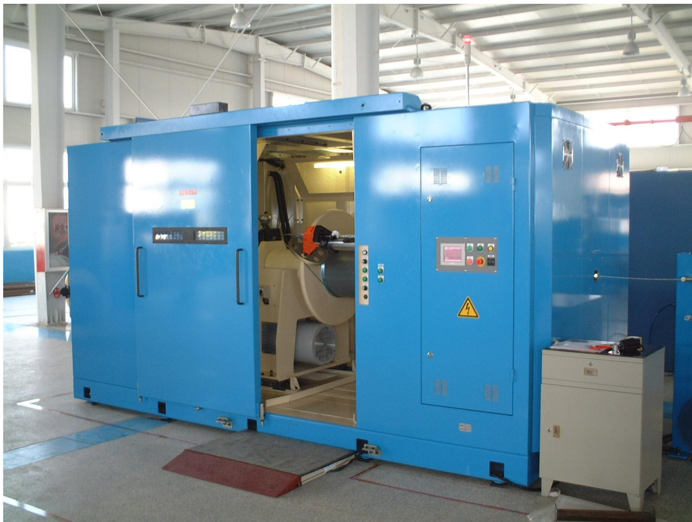
**High performance single twist cabler designed specifically for processing four pair category cables (CAT 6, 6E, 7).**
